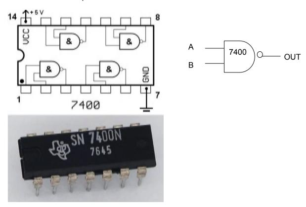
Construct the circuit with an LS7400 2-INPUT POSITIVE NAND GATE. Verify the Truth table. Is it correct?
